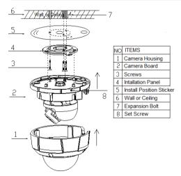
Step one: Measure the height of installation on wall and mark the holes positions.
